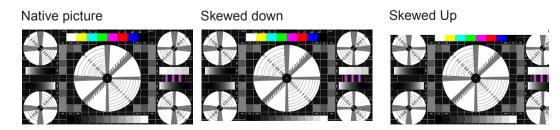
It is recommended that when adjusting the image, the horizontal total should be adjusted before the horizontal phase. However, if the image still flickers even after you have adjusted both, try lowering the image noise.
